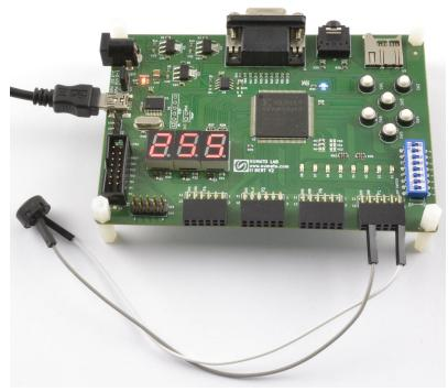
Figure 6-4 Attaching the buzzer to the Elbert 2.
