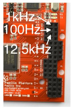
Figure 8-2 Generating multiple frequencies on the Papilio One.
